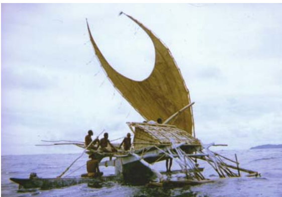
Seafaring in the Polynesian Outliers. Fig. 4 Te puke type voyaging canoe from Taumako island under sail on open sea.
